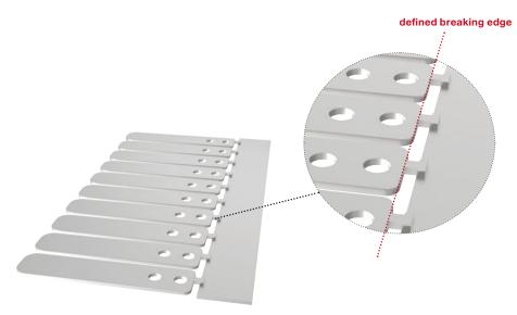
As shown in the picture, a metal strip (carrier plate) was produced on a side with a connection bridge to the single part. You see that it is also important to use the 3-side macro-joint connection.
