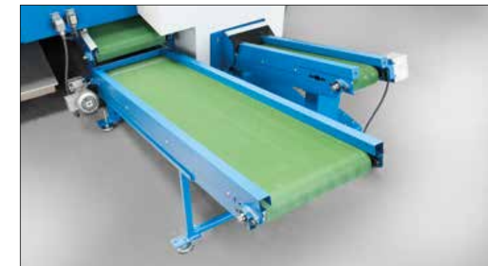
Double conveyor to unloading point
