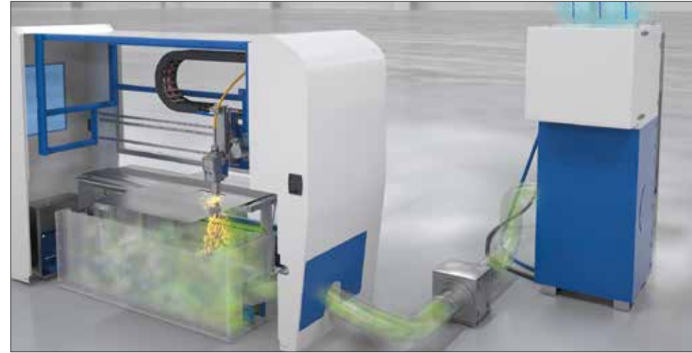
Dust collection for FiberLaser
