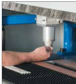
Nozzle change at Laserhead
