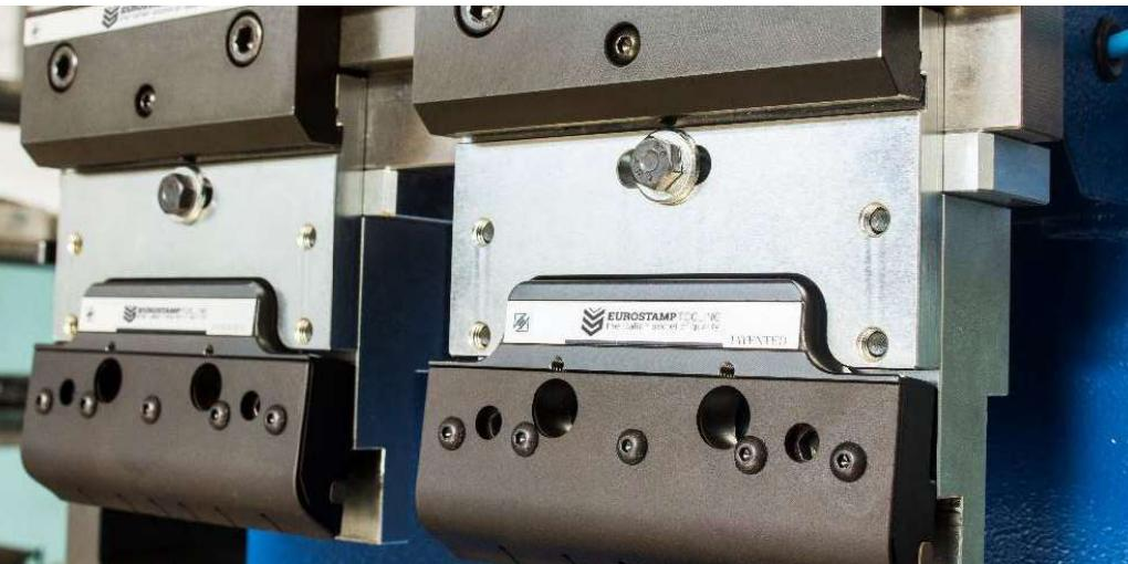
Upper pneumatic clamping system made up of:
