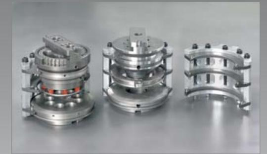
Quick change tool cassettes hold the punch, die and stripper and are set off-line so as not to limit machine run time.
