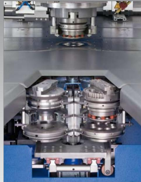
8 station tool carousel with cassettes that hold punch, die and stripper or Revotool head with 4, 6 or 8 tools.
