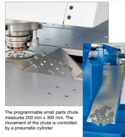
The programmable small parts chute measures 200 mm x 300 mm. The movement of the chute is controlled by a pneumatic cylinder.
