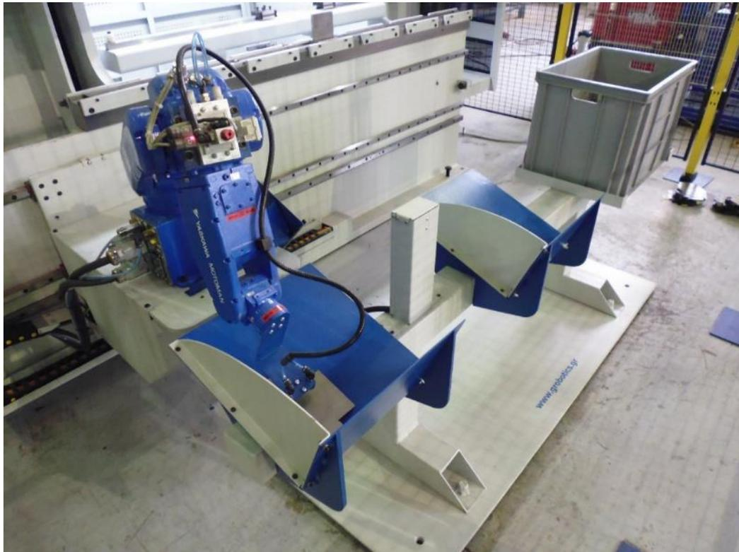
Any Press Brake with RoboBend option can be equipped with Multiple Picking Stations upon request.
