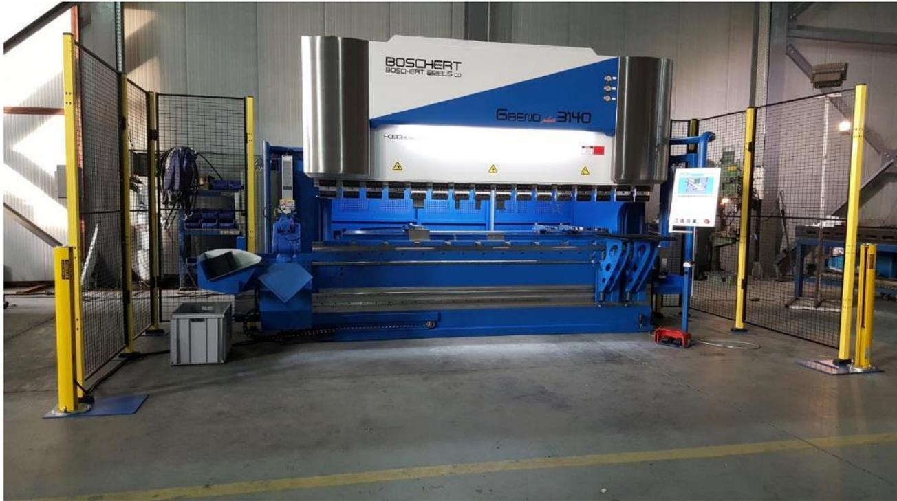
The aim of the safety fence is to ensure the safe working of the system and is certified with CE
