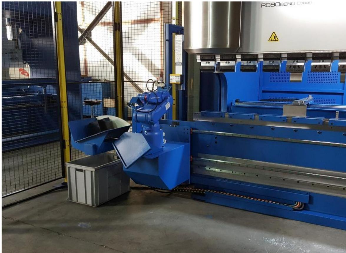
When operations are performed in manual bending the robot is on parking position so that the operator can use the complete length of the press brake
