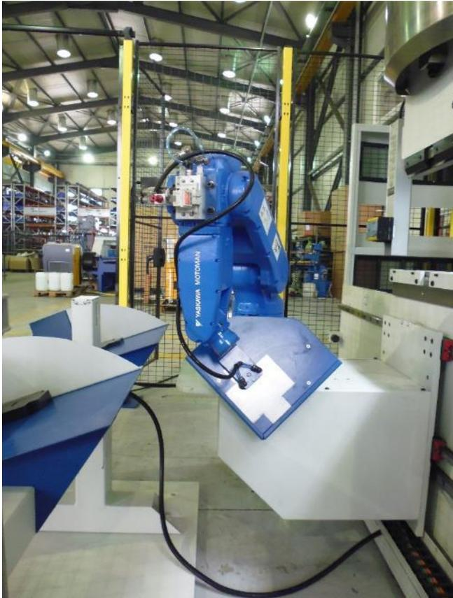
Process of reference of the sheet metal before the bending sequence
