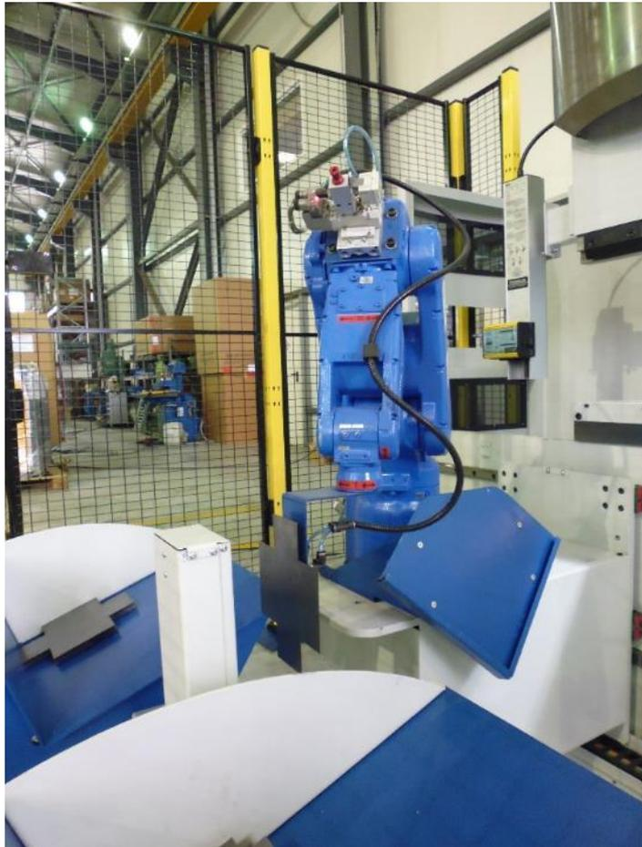
Thickness measurement ensures that the robot holds only one sheet metal during the bending phases
