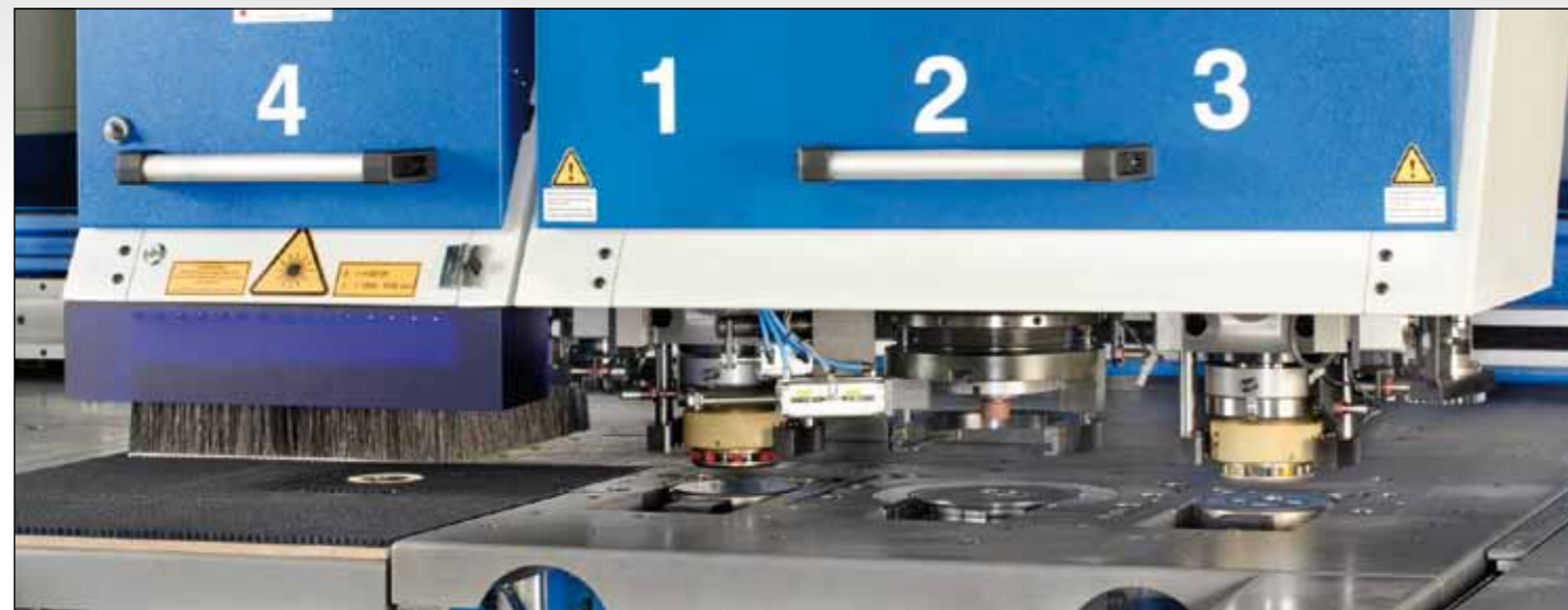
CombiLaser TRI 3-head punching machine with 2xRevotool (head 1 + 3) and rotation / index (head 2)
