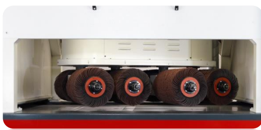
Model 42-Series-1350-WWRbW; 2 x debavurare + rotunjirea muchiiilor + Finisarea suprafetei
