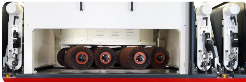
Model 42-Series-1350-WWRbW; 2 x debavurare + rotunjirea muchiiilor + Finisarea suprafetei
