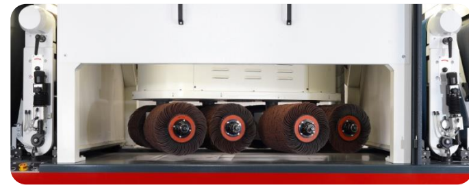
Model 42-Series-1350-WWRbW; 2 x debavurare + rotunjirea muchiiilor + Finisarea suprafetei
